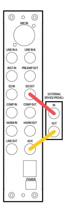
**EXAMPLE 1 (left)** - Re-arranges the signal path to put the LIMITER before the EQ.
